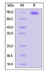
Cynomolgus OSMR, His Tag on SDS-PAGE under reducing (R) condition. The gel was stained with Coomassie Blue. The purity of the protein is greater than 95%.
