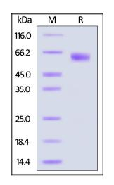
HSV-2 (HG52) Glycoprotein E, His Tag on SDS-PAGE under reducing (R) condition. The gel was stained with Coomassie Blue. The purity of the protein is greater than 95%.
