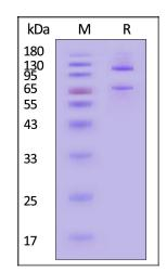
Cynomolgus Complement C5, His Tag on SDS-PAGE under reducing (R) condition. The gel was stained with Coomassie Blue. The purity of the protein is greater than 95% (With <u>Star Ribbon Pre-stained Protein Marker</u>).
