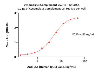
Immobilized Cynomolgus Complement C5, His Tag (Cat. No. CO5-C52Hx) at 2  $\mu$ g/mL (100  $\mu$ L/well) can bind Anti-C5a (Human IgG1) with a linear range of 0.4-6 ng/mL (QC tested).
