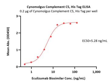
Immobilized Cynomolgus Complement C5, His Tag (Cat. No. CO5-C52Hx) at 2  $\mu$ g/mL (100  $\mu$ L/well) can bind Eculizumab Biosimilar with a linear range of 0.5-31 ng/mL (Routinely tested).
