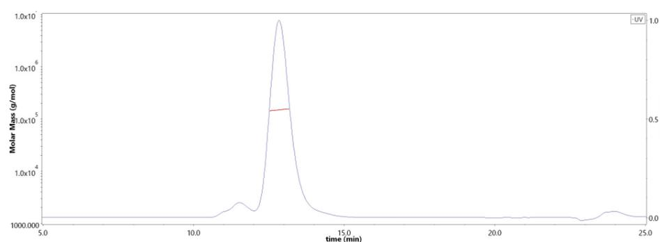
The purity of Mouse CD155, Mouse IgG2a Fc Tag (Cat. No. CD5-M5254) is more than 90% and the molecular weight of this protein is around 130-160 kDa verified by SEC-MALS.
