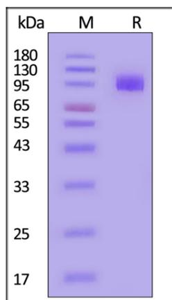
Mouse CD155, Mouse IgG2a Fc Tag on SDS-PAGE under reducing (R) condition. The gel was stained with Coomassie Blue. The purity of the protein is greater than 95% (With [Star Ribbon Pre-stained Protein Marker](#)).
